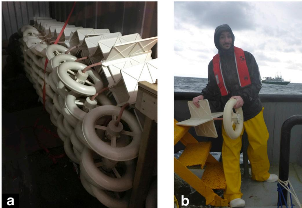
FIG. 20. LASER experiment: (a) 70 CARTHE drifters fully assembled occupy about  $5\text{ m} \times 1\text{ m} \times 1\text{ m}$  along the wall of a container. (b) A graduate student waiting for the signal to launch a drifter off the boat in coordination with the other ship, R/V *F. G. Walton Smith*, in the background.
